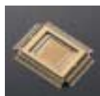
Dolby Digital and DTS decoding LSI (Yamaha Original YSS-918)
