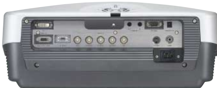
DPX-1000 connection panel offers INPUT A (G/Y, B/Pb/Cr, HD/SYNC and VP), INPUT B (RGB/YPsPr/YCbCr), DVI, S-video input and composite video input terminals, remote control IR Code input/output, RS-232C serial interface, and +12V trigger output terminal.
