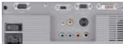
LPX-500 connection panel offers component video (RGB) input (D Sub), component video (RGB) RCA input, S-video input, composite video input and digital RGB input terminals, RS-232C serial interface, and +12V trigger output terminal.
