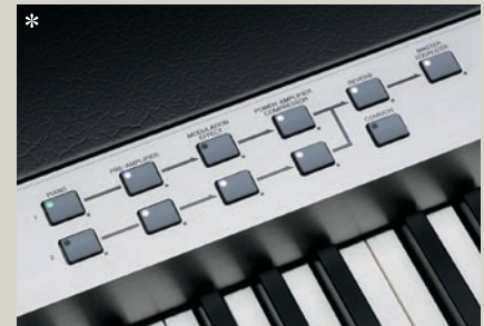
▲ Picture ③ The four blocks that are used to create the CP1 tones are displayed in order through the use of buttons. The piano block consists of the PIANO and PRE-AMPLIFIER sections. It is followed by the MODULATION EFFECT, POWER AMPLIFIER/COMPRESSOR, and REVERB blocks. At the end is the MASTER EQUALIZER. When a button's indicator is lighted, it means that the corresponding block is on.
