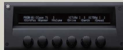
▲ Picture ⑧ The six optimum parameters for changing the tone are pre-assigned to the knobs at the bottom of the screen (these parameters can be changed freely). For Preset-B-1, "Case 71," in the picture, the following parameters are assigned to the six knobs in the center of the panel: the hammer striking point (StrkPos), hammer hardness (Hammer), output volume (Volume), power amp distortion (Drive), vibrato depth (Depth), and speed (Speed).
