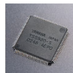
Yamaha's Exclusive YSS-930 32-Bit Floating-Point Quantization LSI
