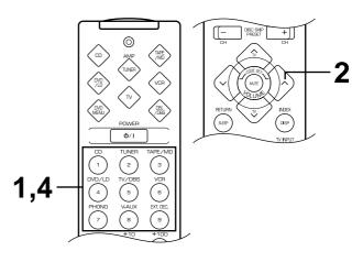
4 When a tape deck or MD recorder is being used for recording, you can monitor the sounds being recorded by pressing **TAPE/MD MON / EXT. DECODER** on the front panel or **TAPE/MD** on the remote control transmitter so that the "TAPE/MD MON" indicator lights up on the display.
