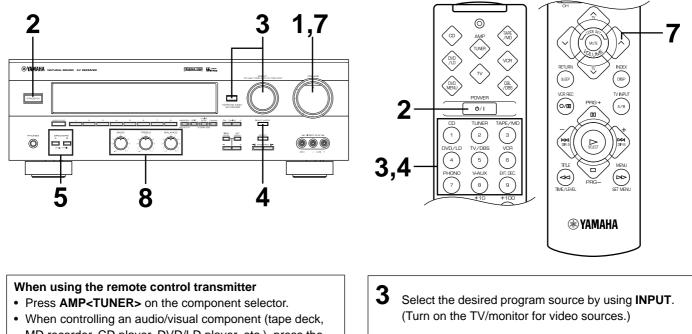
When controlling an audio/visual component (tape deck, MD recorder, CD player, DVD/LD player, etc.), press the button on the component selector, TAPE/MD, CD, DVD/LD, etc., for the component you want to control. (See "SETUP CODES" on page 53.)
