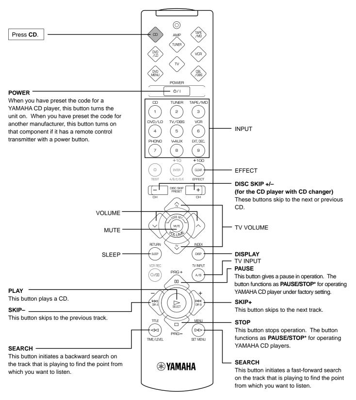
\* PAUSE/STOP function ... Press the button once to give a pause in operation and once more to stop operation.
