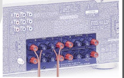
**Connect Main Speakers** Unplug receiver before proceeding. Identify "Front" or "Main" speaker terminals on receiver. Connect left main speaker wire to left main terminals and right main speaker wires to right main terminals as shown. Positive (+) side of the wire with white stripe attaches to red terminal. Negative (-) side attaches to black terminal.
