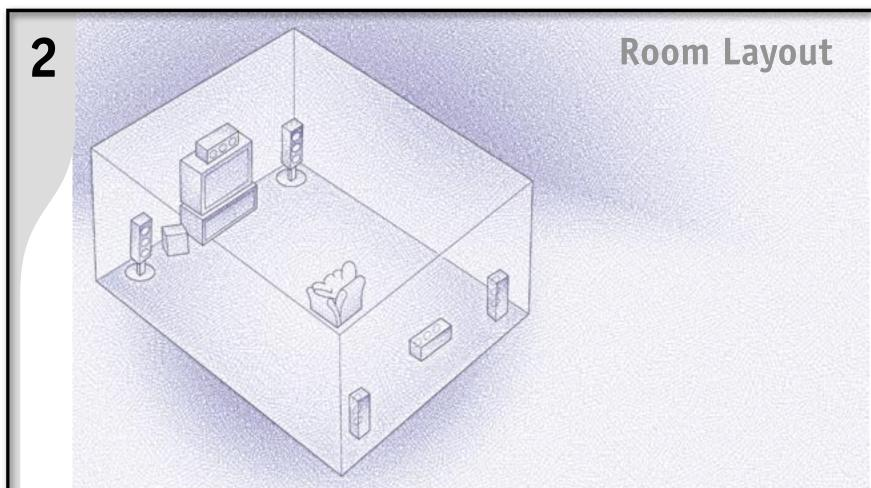
**Speaker Placement** After assembly of the speakers place them so they appear in the approximate positions as shown in the diagram above.
