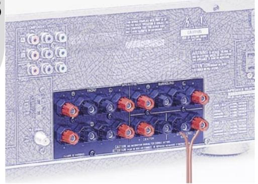
**Connect Rear Center Speaker** Identify Rear Center speaker terminals on receiver. Connect rear center speaker wire to rear center terminals as shown. Positive (+) side of the wire with white stripe attaches to red terminal. Negative (-) side attaches to black terminal.
