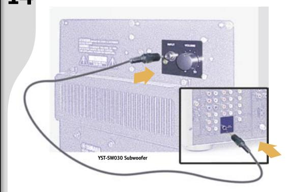
**Connect RCA Cable** Connect RCA cable **(8)** to subwoofer. Set subwoofer VOLUME control to half-way mark and POWER to OFF. Connect RCA cable to receiver from subwoofer.
