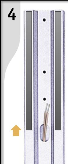
Thread Speaker Wires Cut speaker wire 4 to appropriate lengths for all speaker connections and set aside. Place each long stand upright on its base. Thread main speaker wire through oval opening on stand and pull through opening on underside of base. Pull wire all the way through leaving extra length near oval opening as shown. Apply non-skid pads (14) on stands.
