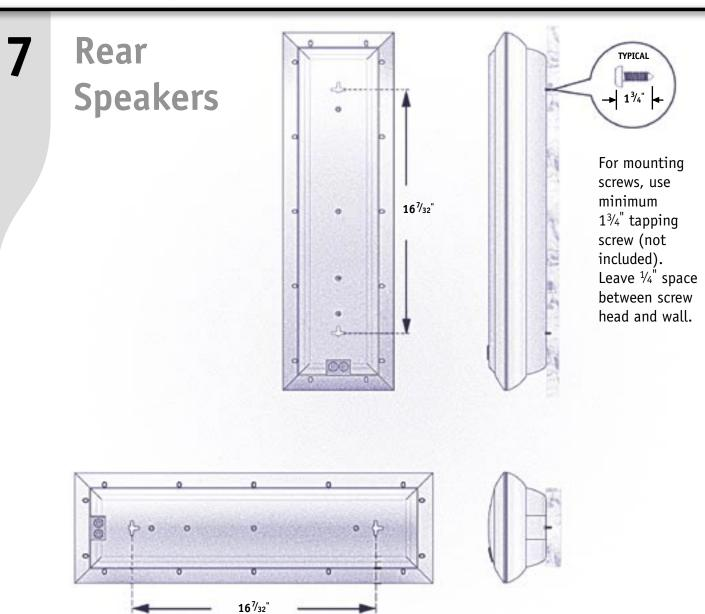
**Mount Rear Speakers and Rear Center Speaker (Optional)** Fasten mounting screws into a firm wall or wall support as shown. Hang the keyholes on the back of the each of the speakers ② on the protruding screws. Attach speaker wire as shown in Step 6.
