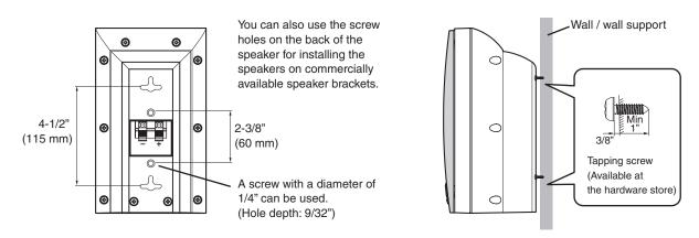
When using speaker brackets to mount the speakers on a wall or celling, it is strongly recommended that safety wire, which may be included with the bracket, be used between the speaker and the bracket to prevent the speaker from falling.
