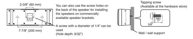
When using speaker brackets to mount the speakers on a wall or celling, it is strongly recommended that safety wire, which may be included with the bracket, be used between the speaker and the bracket to prevent the speaker from falling.
