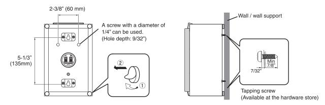
When using speaker brackets to mount the speakers on a wall or ceiling, it is strongly recommended that safety wire, which may be included with the bracket, be used between the speaker and the bracket to prevent the speaker from falling.
