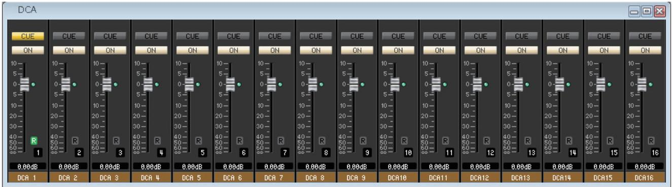
In this window you can view and edit the parameters of DCA (Digital-Controlled Amplifier) groups 1–16.
