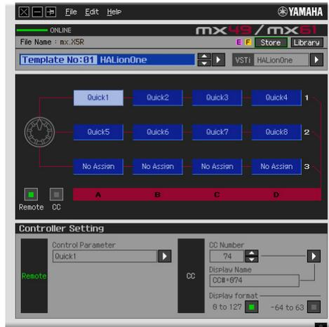
**NOTE** If data transfer in the Auto Sync window fails even when the MX49/MX61 and computer are connected properly, make sure to set the “MIDI IN/OUT” parameter to “USB” and the Device Number parameter to “1” or “All” in the Utility MIDI display on the MX49/MX61.
