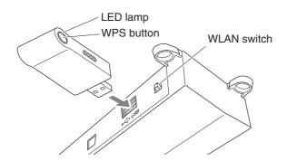
3 Set the WLAN switch on the rear of the switch box to "AP."
