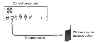
(For upright pianos) Connect the wireless router (access point) to the LAN port on the inlet box using an Ethernet cable.
