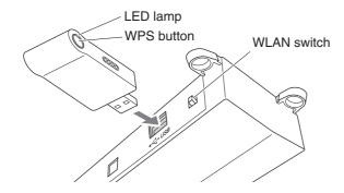
Check that the WLAN switch on the rear of the switch box is set to "RT."
