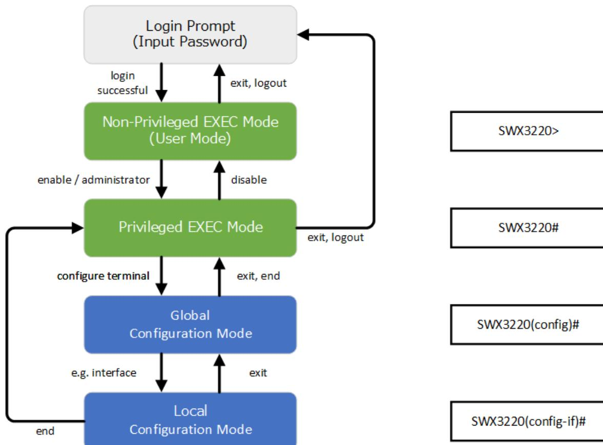
The basic commands related to moving between command input modes are described below. For commands that move from global configuration mode mode to individual configuration mode, refer to "individual configuration mode."
