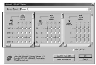
You can change the I/O assignment of the computer's output port and the UX256's output port. The left column shows the computer's output ports (OUT 1-16), and the top column shows the UX256's output ports (1-16). With the default settings, ports with the same number are connected to each other. However, you can change this setting by checking the check boxes.
