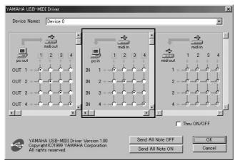
You can change the I/O assignment of the computer's input port and the UX256's input port. The left column shows the computer's input ports (IN 1-8), and the top column shows the UX256's input ports (1-8). With the default settings, ports with the same number are connected to each other. However, you can change this setting by checking the check boxes.
