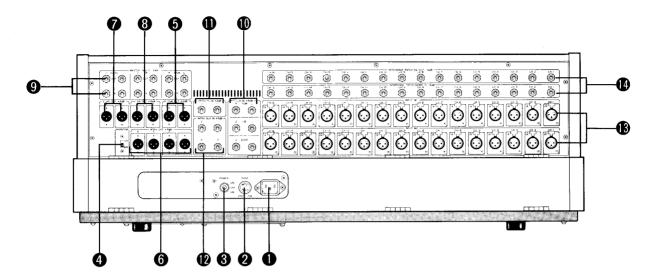
NOTE: All XLR connectors in the M916 are wired as follows: pin 2=signal high, pin 3=signal low, pin 1=shield.
