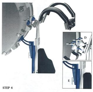
TO ADJUST THE HEIGHT OF THE BASS DRUM, LOOSEN THE  $T ext{-}BOLT$  (E) AND MOVE THE MONOPOSTO SLIDER MUNTIL YOU REACH THE DESIRED HEIGHT. YOU CAN ALSO INVERT THE MONOPOSTO SLIDER MONOPOSTO SLIDER TO LOCK YOUR POSITION IN PLACE.
