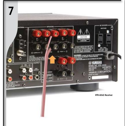
**Connect Center Speaker** Positive (+) side of the wire with white stripe attaches to (+) terminal. Negative (-) side attaches to (-) terminal.
