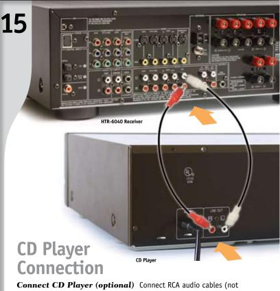
**Connect CD Player (optional)** Connect RCA audio cables (not included) to "CD" terminals on receiver as shown. If your CD Player has digital output terminal, connect digital cable (not included) to HTR-6040 Receiver Digital Input terminal. See your HTR-6040 Owner's Manual for more information.
