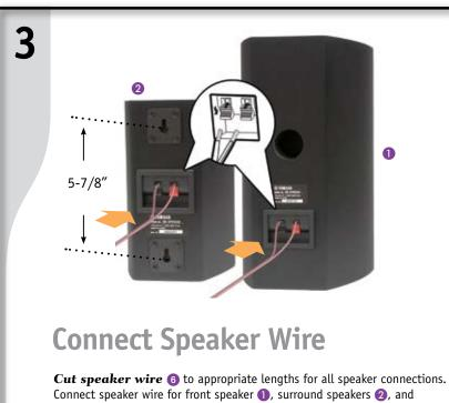
**Cut speaker wire** (a) to appropriate lengths for all speaker connections. Connect speaker wire for front speaker (1), surround speakers (2), and subwoofer (3). The positive (+) side of the wire with the white stripe attaches to the red terminal. The negative (-) side attaches to the black terminal. (See your HTR-6040 Owner's Manual for more information on
