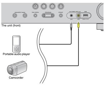
If you select "V-AUX" as the input source by pressing V-AUX, the video/audio played back on the device will be output from the unit.
