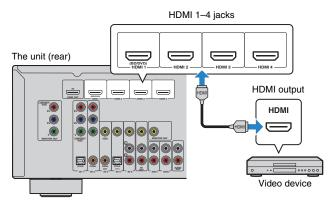
If you select the input source by pressing HDMI 1–4, the video/audio played back on the video device will be output from the unit.
