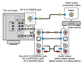
If you select the input source by pressing AV 3–5, the video/audio played back on the video device will be output from the unit.
