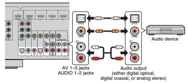
If you select the input source by pressing AV 1–5 or AUDIO 1–2, the audio played back on the audio device will be output from the unit.
