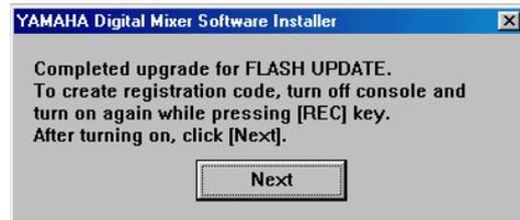
**NOTE:** A different message (see page 10) may appear in various system environments. In this case, quit the installer following the on-screen instruction. Turn off the power to the console, then press and hold down the [REC] button (on the DM1000, the [CLEAR] key) and turn on the power. The console displays “FLASH UPDATE.” Start the installer and repeat Steps 5 through 9. Proceed to Step 14.
