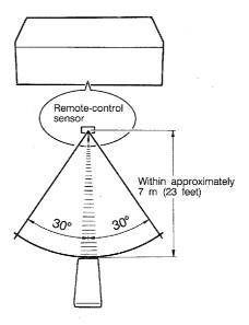
There should be no large obstacles between the remotecontrol transmitter and the main unit.
