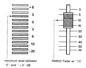
The REC LEVEL control on the deck can be used to optimize the fader setting, as can the level control on the instrument used—in this case the RX15.
