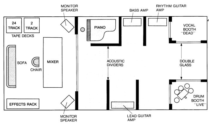
Floor plan of professional multitrack recording studio
