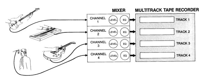
For playback, the multitrack tape recorder's outputs are connected to the mixer's inputs. The mixer's stereo outputs are connected to monitors (speakers). The signal from each track can be set to the left or right stereo outputs, or anywhere in between. For example, the bass recorded on track 1 of the multitrack
