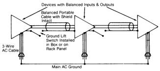
Perhaps the best answer to portable system grounding problems, RFI, EMI, and AC noises, is to develop a versatile grounding scheme. Ground lift switches and adapters, and a portable AC power distribution system allow different grounding techniques to be tried easily and quickly when a problem occurs.
