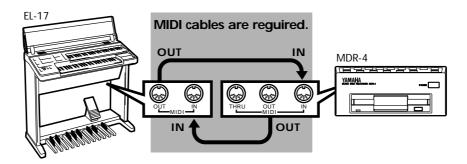
To communicate with each other, the MIDI transmit/receive channels of the external MIDI device must match the receive/transmit channels of your EL-17 since the MIDI channels of the EL-17 are preset to the following numbers.
