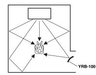
Figure 3. With a sound reflection board installed
