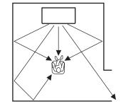
Figure 2. Surround (right) beam is not being reflected because there is no wall.
