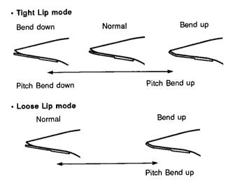
In the WX11 the tight lip mode is the "normal" playing mode, and is selected automatically when the WX11 system power is turned ON. The loose lip mode can be selected simply by holding down the WX11 setup switch while turning on the system power.
