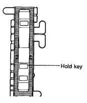
The hold key makes it possible to produce a pedal tone over which other notes can be played. To produce a held tone, simply press the hold key while playing the note to be held. The note will be held even after you release the hold key, and you can play other notes over the held tone in the normal way. To stop the held tone, simply press the hold key while no breath is applied to the mouthpiece (no note is being played).
