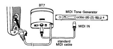
With the BT7 MIDI/Power Pack, the WX11 can be used with the following devices:
