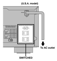
After completing all connections, connect the AC power cord to an AC power outlet. Disconnect the AC power cord if you will not use this unit for a long period of time.
