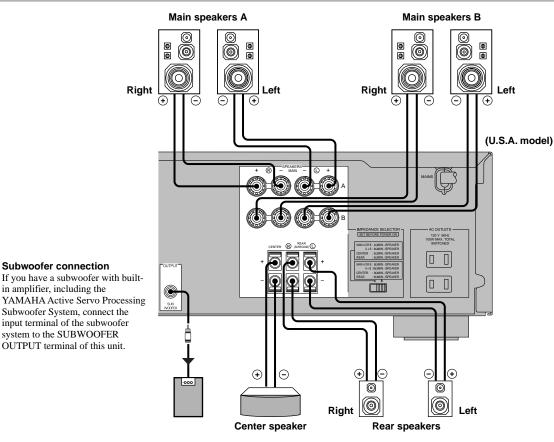
Be sure to connect the right channel (R), left channel (L), "+" (red) and "-" (black) properly. If the connections are faulty, no sound will be heard from the speakers, and if the polarity of the speaker connections is incorrect, the sound will be unnatural and lack bass.
