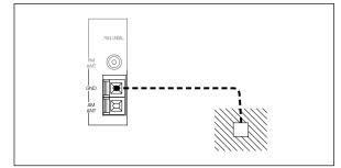
The AM loop antenna can be removed from the stand and attached to a wall, etc. However, note that the reception sensitivity may deteriorate if the antenna is attached to a metal or steel reinforced wall.
