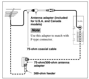
Firmly insert the connector into the FM ANT terminal. The indoor FM antenna is only a simple antenna. For reception with better sound quality, installing the outdoor FM antenna (commercially available) is recommended.
