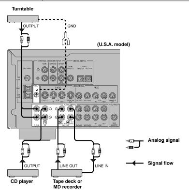
Be sure to connect the right channel (R), left channel (L), input (IN) and output (OUT) properly.
