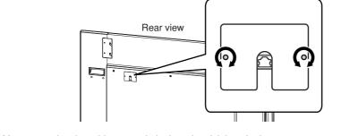
After connecting the cable, reattach the board and tighten both screws to secure it.
