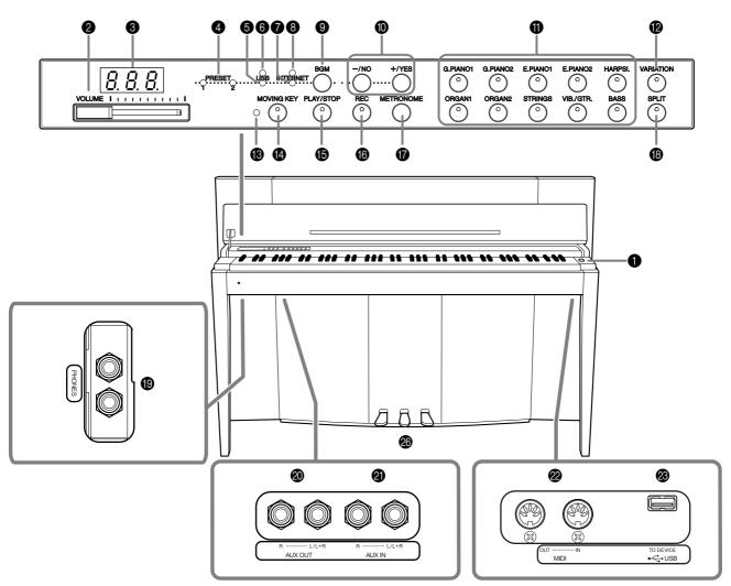
The jacks and terminals on the underside of the instrument as shown here may seem to be in reverse from your perspective in front of the instrument. Make sure when using these to carefully check the names as printed on the panel before making connections.
