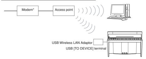
\* Here, "modem" refers to an ADSL modem, optical network unit (ONU) or cable modem.
