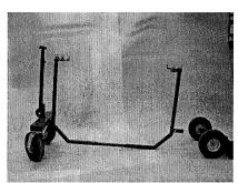
Take bottom frame, C, and either insert A or insert B depending on size of Drum then tighten both set screws on frame C.
