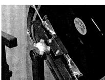
Put drum on carrier with 5/16" bolts with rubber protectors outside lug and between tension rods and drum.
