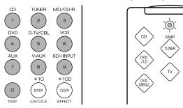
5. To verify the code works, aim the remote control at the television set, press TV, and then press POWER. The television set should turn off. If it doesn't respond, use another code for the same manufacturer and repeat steps 3 through 5.
