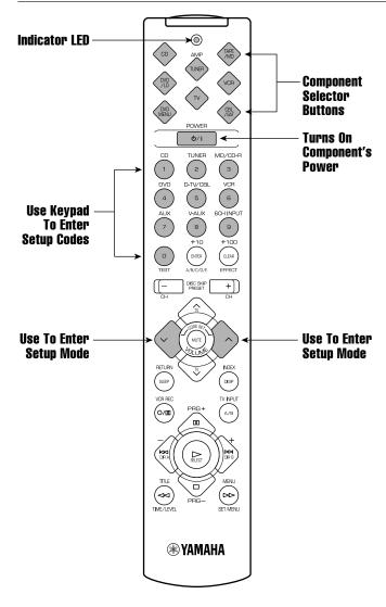
The YHT-18 Home Theater package includes a universal remote control. It comes pre-programmed with factory codes to control your HTR-5440 receiver and most Yamaha audio components. To program other brands of components (i.e., TV, VCR, etc.) or if your Yamaha unit does not respond, you will need to program the remote control with the manufacturer's codes (listed on the back pages of the *HTR-5440 Owner's Manual*).
