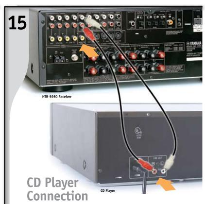
Connect CD Player (optional) Connect RCA audio cables (not included) to "CD" terminals on receiver as shown. If your CD Player has digital output terminal, connect digital cable (not included) to HTR-5950 Receiver Digital Input terminal. See your HTR-5950 Owner's Manual for more information.
