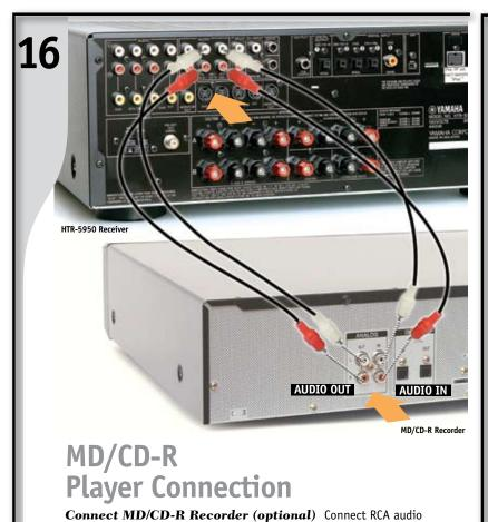
cables (not included) to "MD/CD-R" terminals on receiver as shown.
