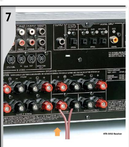
Connect Center Speaker Positive (+) side of the wire with white stripe attaches to (+) terminal. Negative (-) side attaches to (-) terminal.
