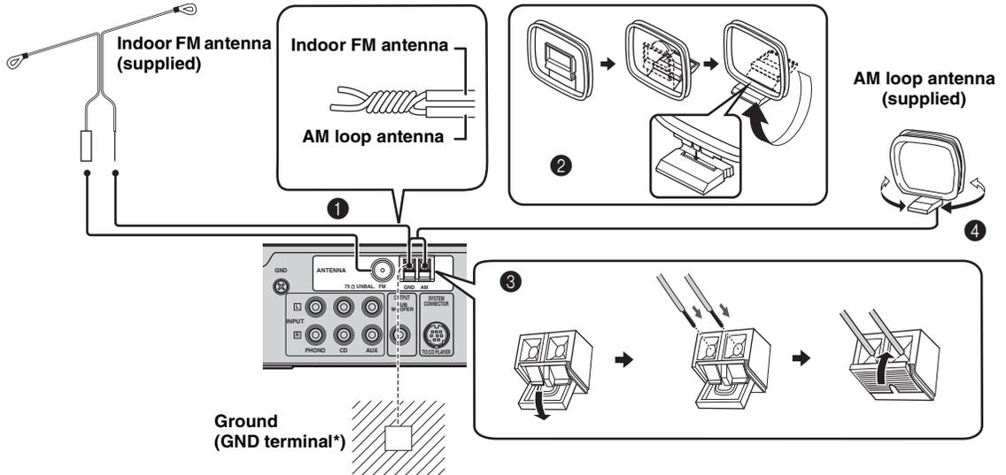
\* For the maximum safety and minimum interference, connect the antenna GND terminal to a good earth ground. A good earth ground is a metal stake driven into the moist earth.
