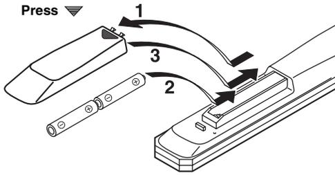
**1** Press the ▼ part and slide the battery compartment cover off.
