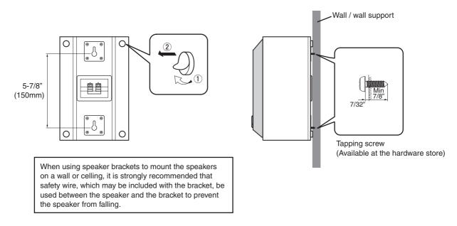
Fasten screws into a firm wall or wall support as shown in the figure, and hang the holes of the mounting bracket on the protruding screws.
