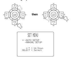
If  $\wedge$  is pressed when AUTO SETUP is selected, or if  $\vee$  is pressed when MANUAL SETUP is selected, SET MENU will be closed. Press  $\wedge$  / $\vee$  to open SET MENU again.
