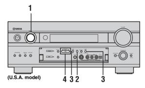
1 Rotate INPUT (or press TUNER on the remote control) to select TUNER as the input source.
