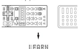
5 Press and hold the button you want to program on the other remote control until "OK" appears in the display window.
