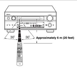
The remote control transmits a directional infrared beam. Be sure to aim the remote control directly at the remote control sensor on the main unit during operation.
