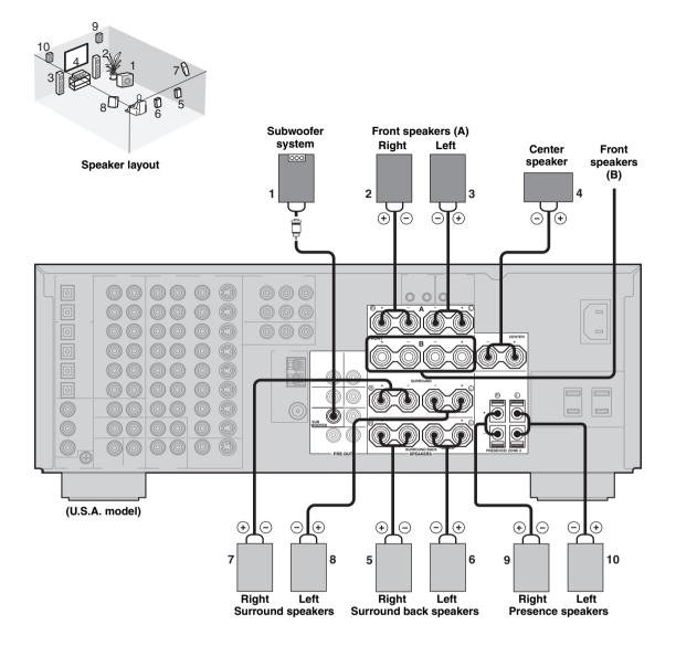
You can connect both surround back and presence speakers to this unit, but they do not output sound simultaneously.
