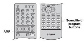
Press AMP to select the AMP mode, then press one of the sound field program buttons repeatedly to select the desired program.
