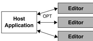
OPT-compatible plug-in software is connected directly to an OPT-compatible host application.
