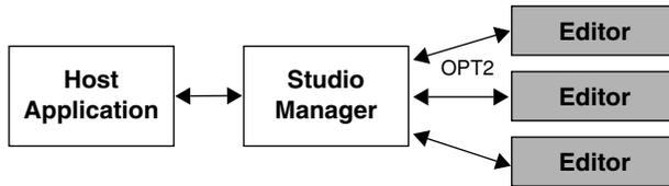
Plug-in software compatible with OPT 2 is indirectly connected to the DAW application compatible with Total Recall, via the Studio Manager.
