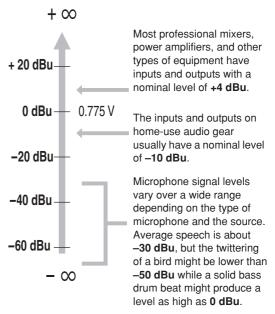
A mixer may be required to handle signals at a wide range of levels, and it is necessary match input and output levels as closely as possible. In most cases the "nominal" level for a mixer's input and outputs is marked on the panel or listed in the owner's manual.
