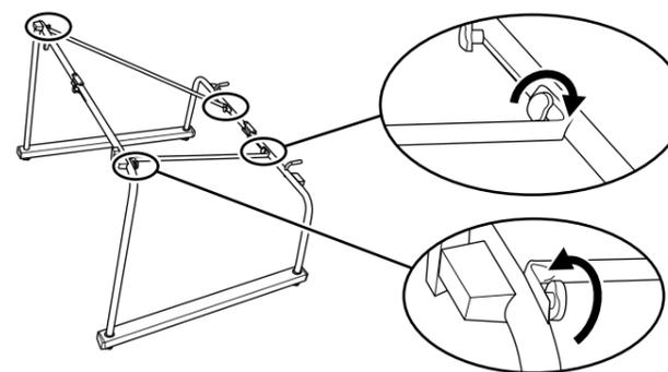
**NOTE** When removing the braces at disassembly, the screws of the braces may hard to loosen. In this case, loosen the screws while moving the braces lightly to the front, back, left and right.
