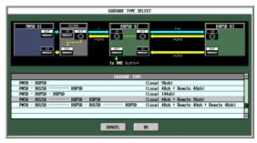
This system cascade-connects one DCU5D and two DSP5D units to the PM5D, adding 96 remotely located monaural inputs.
