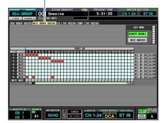
Except for the fact that these settings apply to input channels, the display and operations are the same as in the OUTPUT DCA/GROUP function MUTE GROUP ASSIGN screen. Refer to p.259.
