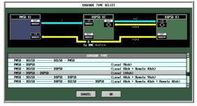
This system cascade-connects two DSP5D units to the PM5D, expanding the number of input channels to 144 monaural input channels.
