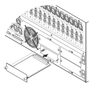
**4** Use the screws included with the card to fasten the card in place. Malfunctions or incorrect operation may occur if the card is not fastened.
