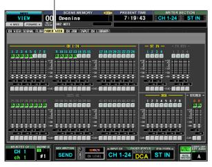
Except for the fact that this screen is for input channels, DCA groups, and STEREO A/B channels, this is the same as the OUTPUT VIEW function FADER VIEW screen. Refer to p.273.
