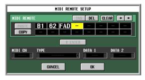
When you click a box in which a hexadecimal value has been input, the range of values that can be interpreted as a valid MIDI message (including that box) will turn red. The lower part of the screen shows the MIDI channel (MIDI CH), message type (TYPE), and data values (DATA 1, DATA 2) for this MIDI message, letting you verify that the appropriate MIDI message has been input.
