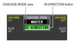
When multiple PM5D units are cascaded, the settings of the CASCADE MODE area specify whether the unit will operate as a cascade master (when "MASTER" is selected) or as a cascade slave (when "SLAVE" is selected).
