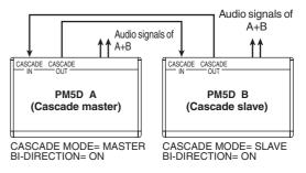
In this state, the SLAVE unit will follow when you operate the MASTER unit. The same mix will be output from both PM5D units.
