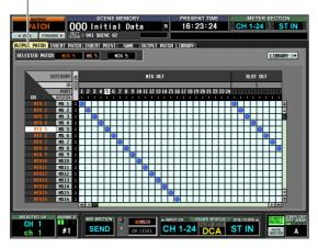
In the OUTPUT PATCH screen you can patch (assign) output channels to output ports. The horizontal direction of the screen shows the output ports (i.e., patch destinations), and the vertical direction of the screen shows the output channels (i.e., patch sources). When the PM5D is in its default state, MIX channels 1–24, MATRIX channels 1–8, and the STEREO A channel are patched to the output channels of slots 1–4 and the 2TR OUT DIGITAL jacks in addition to the
