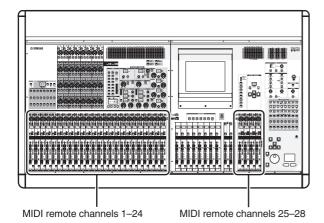
To each controller you can assign a MIDI message consisting of up to sixteen bytes of hexadecimal data. If desired, you can specify that a value within the message varies according to the movement of the controller.
