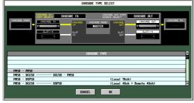
This system directly cascade-connects PM5D units. A maximum of four PM5D units can be connected. Use (2)–(7) to specify the details of the cascade connection.
