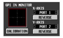
When you specify a GPI IN port, the voltage from that GPI IN port is indicated by a yellow <sup>()</sup> symbol in the GPI IN monitor area. In this case, the horizontal position (X-axis) corresponds to the voltage of the GPI IN port selected in the X-AXIS field, and the vertical position (Y-axis) corresponds to the voltage of the GPI IN port selected in the Y-AXIS field.
