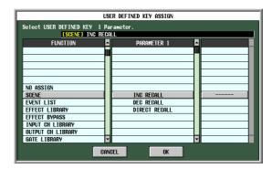
**4** Select the desired function in the FUNCTION column, select parameters in the PARAMETER 1/2 columns, and click the OK button.
