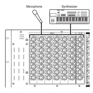
INPUT jacks 1–48 and ST IN jacks 1–4 will accommodate connections ranging from microphones to line level devices.
