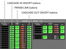
The CASCADE IN and CASCADE OUT ON/OFF buttons specify whether signals of each bus will be transmitted to or received from the cascade-connected external device. These settings are made independently for each bus; MIX buses 1–24, STEREO A bus L/R, STEREO B bus L/R, and CUE bus L/R.
