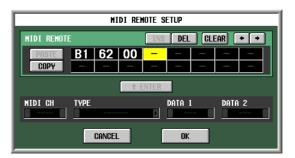
In this window you can input a message by clicking the desired input box to select it (the box will be high-lighted) and turning the [DATA] encoder. You can use the [INC]/[DEC] keys to move the selected position. You can input the following values.
