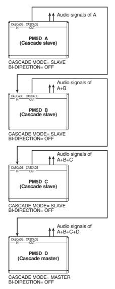
In this state, the SLAVE units will follow when you operate the MASTER unit. The final mix of all signals will be output from the PM5D that is connected last in the chain.
