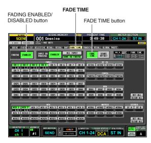
2 In the upper left of the screen, click the FAD-ING ENABLED/DISABLED button to select ENABLED.
