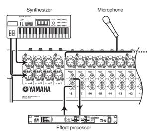
INPUT jacks 1–48 are used mainly to connect microphones or monaural line-level devices. ST IN jacks 1–4 are used mainly to connect stereo line-level devices. Input signal sensitivity, pad on/off, and phantom power (+48V) on/off are controlled from the top panel AD IN section ( $rac{1}{p}$  p.44).
