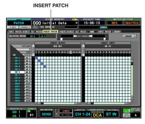
If you want to insert into an output channel, press the OUTPUT [PATCH] key several times to access the OUTPUT PATCH function INSERT PATCH screen.
