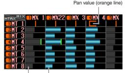
Channels for which the signal sent to the MATRIX bus is turned off (gray bar graph)
