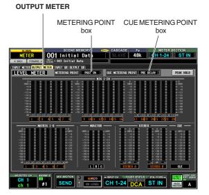
2 To specify the metering point for output channels and MONITOR channels, click the
