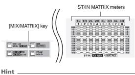
The detection point (metering point) of the signal levels shown in the meters can be changed if desired ( $\Rightarrow$  p.109).
