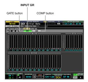
2 Click the GATE button or COMP button to select the parameter that will be displayed. For an explanation of the items shown in the screen, refer to the explanation of the INPUT GR screen (➡ p.233) in the Reference section.
