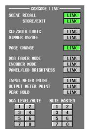
The settings of the CASCADE LINK area select the operations that will be linked when multiple PM5D units are cascade-connected. You can select the following items.
