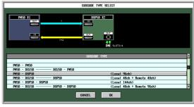
This system cascade-connects one DSP5D unit to the PM5D, expanding the number of input channels to 96 monaural input channels.
