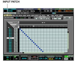
The INPUT PATCH screen is where you can patch (assign) input ports (rear panel input jacks or input channels of I/O cards) to input channels.
