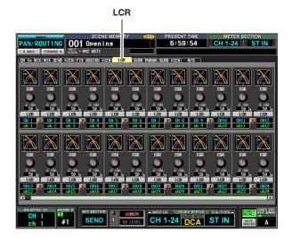
Except for the fact that the send-sources are input channels, the display and operations are the same as in the MATRIX/ST function LCR screen. Refer to p.267.
