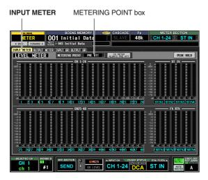
2 Click the ▲ / ▶ buttons at the left and right of the METERING POINT box to choose one of the following metering points.
