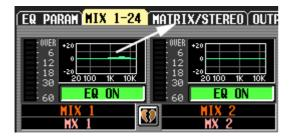
You can also copy settings between the eight-band EQ of a MIX channel or STEREO A/B channel and the four-band EQ of a MATRIX channel. In this case, only the LOWER four bands will be copied for MIX channels or STEREO A/B channels.
