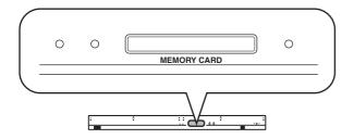
You can use PCMCIA Type II PC flash ATA cards, or CompactFlash media inserted in a PC card adaptor. (In either case, media with a power supply voltage of 3.3V or 5V is supported.) Normally, these cards are sold in an already-formatted state. This means that you won't need to format them before using them with the PM5D. If you do need to format a card, use a computer or other external device to format the card in FAT16 format.
