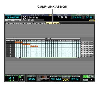
Except for the fact that these settings apply to input channels, the display and operations are the same as in the OUTPUT DCA/GROUP function COMP LINK ASSIGN screen. Refer to p.261.
