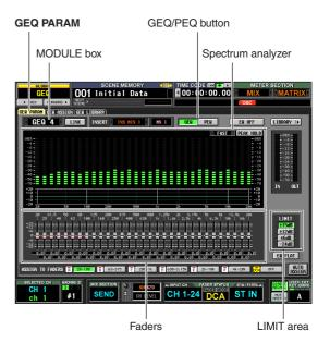
2 Click the < / > buttons at the left and right of the MODULE box to select the GEQ module you want to operate.
