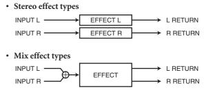
If a signal is assigned to only one input of an effect, it will be processed as mono-in/stereo-out regardless of whether a Stereo effect type or Mix effect type is selected.
