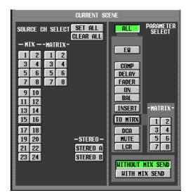
• When PASTE MODE = DCA, GEQ, EFFECT Select DCA groups, GEQ modules, and internal effects.
