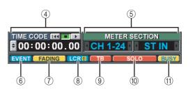
④ PRESENT TIME, TIME CODE, CASCADE/Fs Click this area to cycle through the following three items of information. This is linked with the UPPER PART DISPLAY setting in the PREFERENCE 2 screen (UTILITY function). **Global** functions
