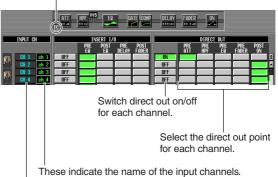
The "D" symbol indicates the direct out point for the channel at which the cursor is located
