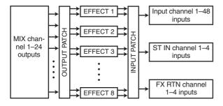
Alternatively, you can insert an internal effect into a channel by assigning the input/output of the internal effect to the insert-out/insert-in of the desired channel.
