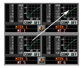
You can also copy compressor settings between the MIX 1-24 screen and the MATRIX/STEREO screen. First drag the mini-graph over the MIX 1-24 tab or MATRIX/STEREO tab in the screen (the screen will switch). Then drag and drop the mini-graph onto the desired channel, and a message will ask you to confirm the copy operation.
