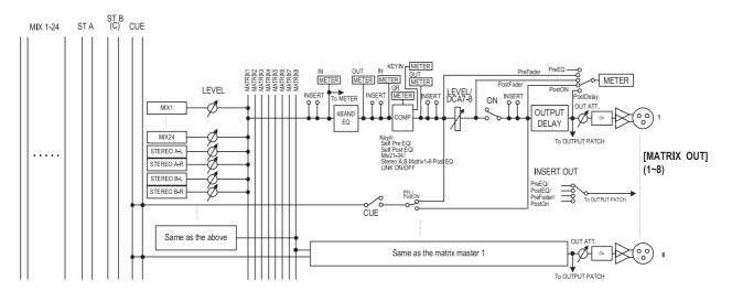
• 8 BAND EQ (8 band equalizer) (MIX channels and STEREO A/B channels)
