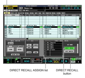
In the SCENE screen you can use the DIRECT RECALL ASSIGN list shown in the lower middle of the screen to assign scene numbers to the SCENE MEM-ORY [1]–[8] keys.
