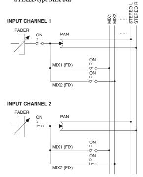
If the send-destination MIX bus is set to FIXED mode, the MIX encoders have no effect; the signal can only be switched on/ off by the MIX [ON] key.
