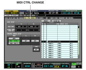
In the MIDI CTRL CHANGE screen you can select the port used to transmit/receive MIDI messages, and how control changes will be transmitted and received. If control change 1–119 is selected as the transmission/ reception method, you can assign the desired event to each control number. **3** In the CONTROL CHANGE SETUP area at the left of the screen, you can select the way in which control changes will be transmitted and received, and switch reception and transmission on/off.
