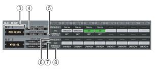
③ Slot number / Card type This area shows the type of digital I/O card installed in slots 1–4.
