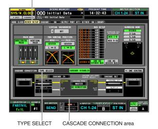
In the CASCADE CONNECTION area located at the bottom of the screen, click the TYPE SELECT button to access the CASCADE TYPE SELECT window.
