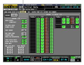
In this combination you can enable/disable buses used for transmission/reception in the cascade connection, and select the operations that will be linked when multiple PM5D units are cascade-connected.
