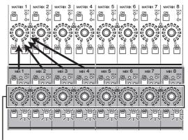
Use the encoders of the MIX section to adjust the send levels
