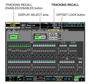
2 In the upper left of the screen, click the TRACKING RECALL ENABLED/DISABLED button to make it indicate ENABLED.
