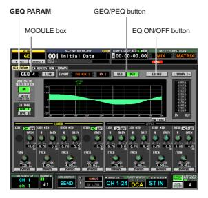
In the MODULE box, click the left/right / buttons to select the GEQ module that you want to operate.
