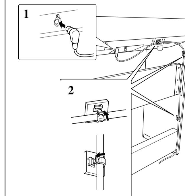
**3 Connect the pedal cord plug to the keyboard.**
