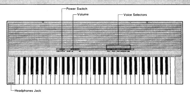
Keyboard-61 Keys (C1-C6) Voice Section -Piano 1, 2, 3, Harpsichord, Vibes Effects and Controls -Damper, Volume, Pitch Other Fittings-Headphone Jack, AUX OUT (Left/Right) Jacks, DC In Jack, Damper Jack, Power Switch, Power-on Light, Damper Pedal FC-5, Music Rest, Dust Cover Amplifier -2W Speaker-12cm (4-3/4") (4Ω)
