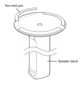
3 Pass the speaker cable through the speaker stand from the under side of the speaker stand.
