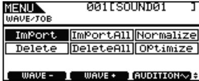
Whenever you press the [F3] button (EXECUTE) on any of the pages accessed via the Wave/Job page, a confirmation panel will be displayed. If you decide to proceed with the corresponding operation, the content of the DTX700's internal memory will be permanently affected.
