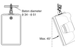
Note In order to prevent the unit from falling down, attach the safety wire as shown in the illustration.
