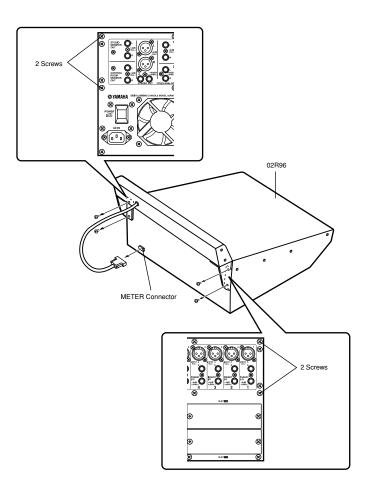
**4.** Remove the screws indicated in the illustration below: 7 screws from the left side, 7 screws from the right side, 7 screws from the front, and 7 screws (or 5 screws, if 2 were already removed at Step 3) from the rear.
