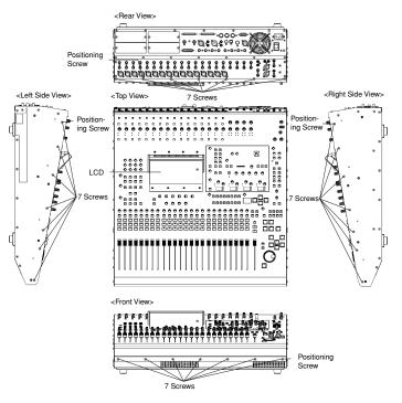
5. Hold onto the LCD, and lift up the rear of the control panel.
