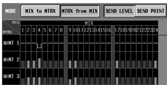
② **SEND LEVEL (发送电平) / SEND POINT (发送点)**
