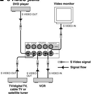
If your video component has "S" (high-resolution) video jacks, they can be connected to this unit's S VIDEO jacks. Otherwise, connect the composite video jacks of your video component to this unit's composite video jacks.
