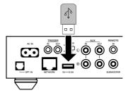
While holding down ▶ (CONNECT) on the front panel, plug the power cable to the AC wall outlet.
