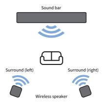
The sound bar and wireless speakers are connected wirelessly for communication between them. For that reason, when using these products for the first time, the respective device information of the sound bar and wireless speakers needs to be registered to one another.
