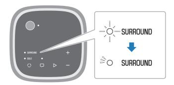
If you only want to connect one wireless speaker, the registration procedure is complete. Proceed to install the wireless speaker.
