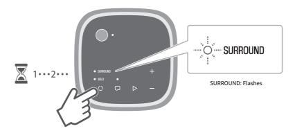
In the next step, operate the controls of the sound bar. Operate the controls of the sound bar within two minutes after the wireless speaker has entered the registration wait status.
