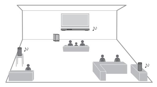
Point the sound bar remote control at the sound bar and press the ALL key to switch to ALL mode.
