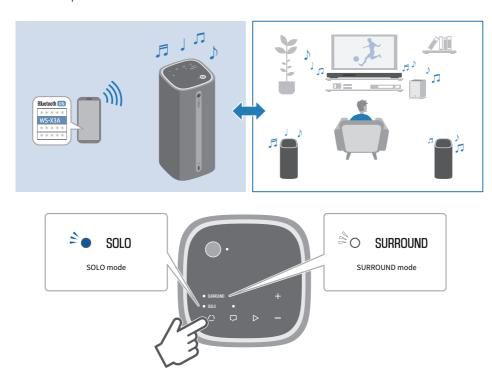
For details on operating in SOLO mode, refer to the wireless speaker User Guide.
