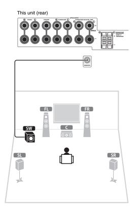
Use an audio pin cable to connect the subwoofer
