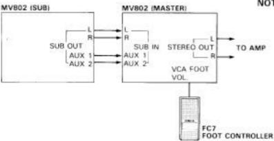
Refer to the BLOCK DIAGRAM on page 8 for details on signal routing in cascaded operation.
