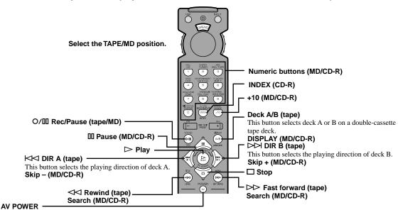
(Tape) This button turns on the tape deck that has a remote control with a power button if you have set up the code for another manufacturer. (MD) This button turns on the MD recorder that has a remote control with a power button if you have set up the code for another manufacturer. (CD-R) This button turns on the CD recorder that has a remote control with a power button if you have set up the code for another manufacturer.
