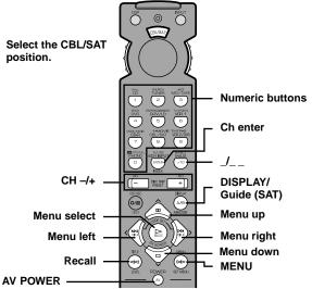
This button turns on a cable TV/satellite tuner that has a remote control with a power button if you have set up the code for your cable TV/satellite tuner.
