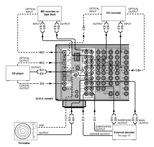
indicates signal direction indicates left analog cables indicates right analog cables indicates optical cables ·**-**·(C)indicates coaxial cables
