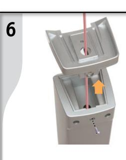
Turn Speaker Stand Right-Side-Up Remove screw that holds adapter in, carefully set aside, then remove adapter from speaker stand.
