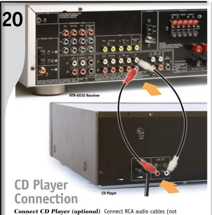
Connect CD Player (optional) Connect RCA audio cables (not included) to "CD" terminals on receiver as shown. If your CD Player has digital output terminal, connect digital cable (not included) to HTR-6030 Receiver Digital Input terminal. See your HTR-6030 Owner's Manual for more information.
