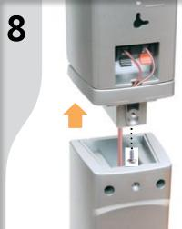
Attach Adapter to the Speaker using the supplied screw O.
