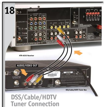
Connect DSS/Cable/HDTV Tuner Box (optional) Connect RCA audio/video cables (not included) and optional optical cable (not pictured)
