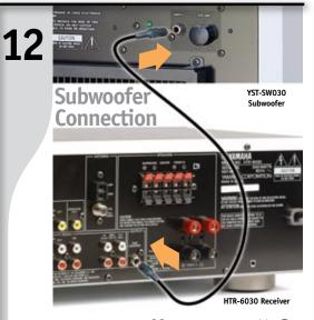
Connect RCA Cable Connect RCA cable 9 to subwoofer 4. Set subwoofer VOLUME control to half-way mark and POWER to OFF. Connect RCA cable to receiver from subwoofer.
