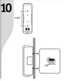
**Mounting Speakers** to Wall (Optional) Fasten mounting screws into a firm wall or wall support. Leave 7/32 in. between head and wall. Hang the keyholes on the speaker backs on the
